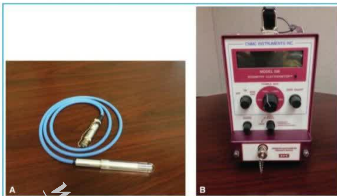
Figure 6.9. Photographs of the ion chamber and electrometer. A: PTW Model TN30013 ion chamber; B: CNMC Model 206 electrometer.
